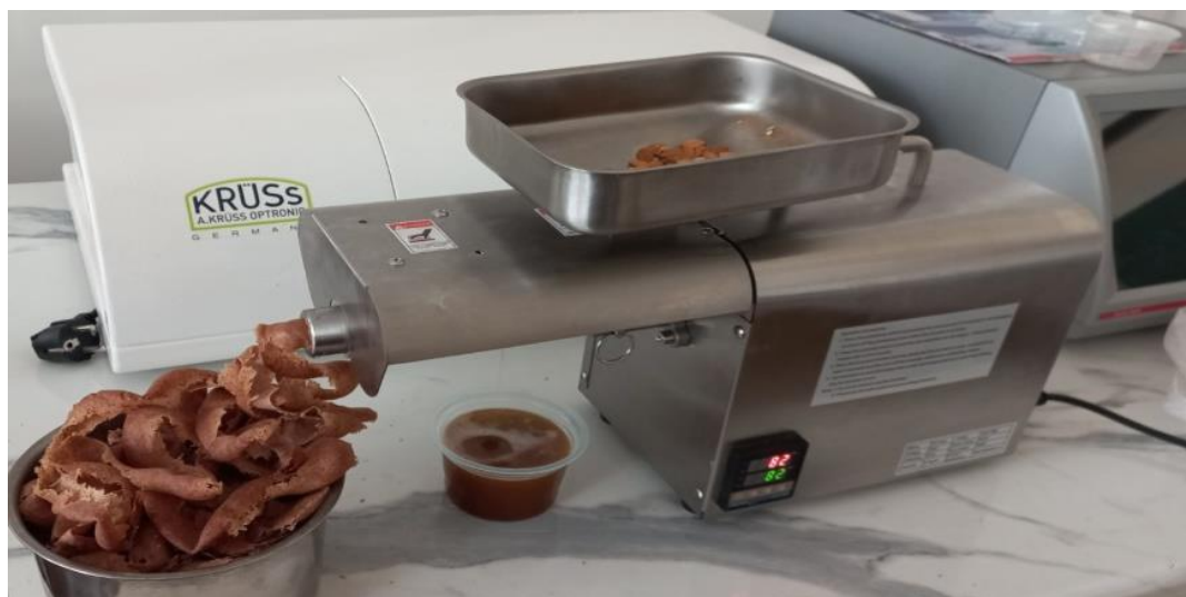
Figure-2. The process of extracting oil from peach kernels
